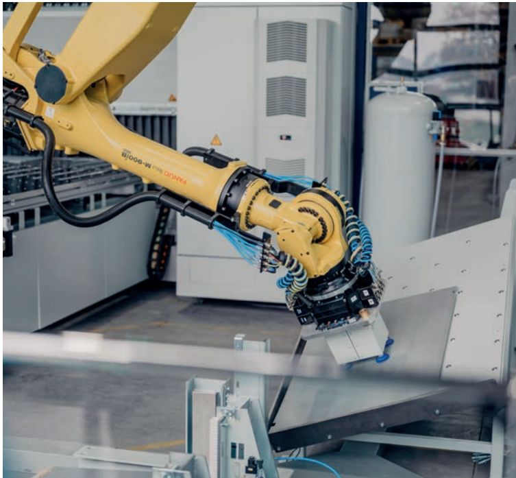
Fanuc robot used: The sheet metal is pre-centered on the deposit table and sucked in by a vacuum unit
