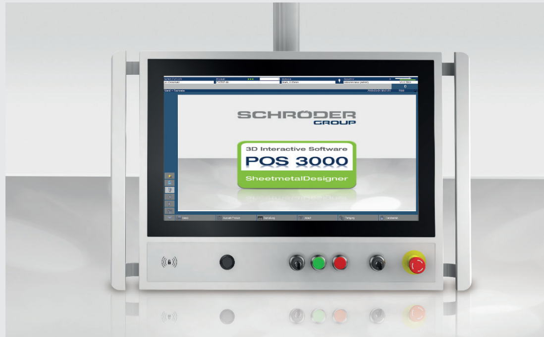
A human-machine interface the way it should be: Folding machines from Schröder receive their instructions via touch display panels.
