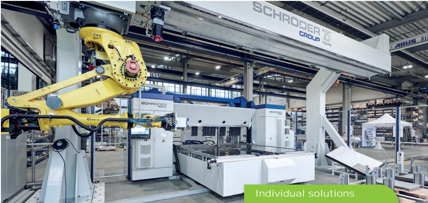
Front view of robot handling system with integrated motorized folding machine MAK 4 Evolution UD: Working length x sheet thickness 3,200 mm x 6.0 mm
