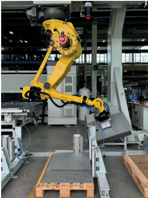
Fanuc robot used: The sheet metal is sucked in by a vacuum unit
