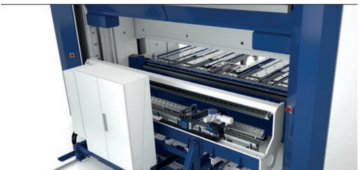
Picture above: A rotating plate controlled by high-precision camera systems aligns the sheet in the machine and transports it fully automatically to the bending line.
