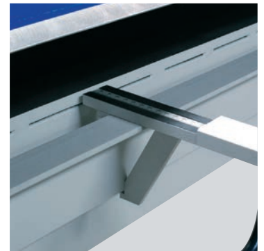
Back gauge- and sheet support system up to 500 mm (BAM 1000) or 750 mm (BAM 2000)
