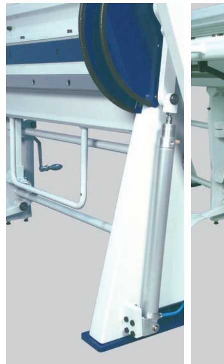
The pneumatic bending support is controlled by a finger lever on the folding beam handle.
