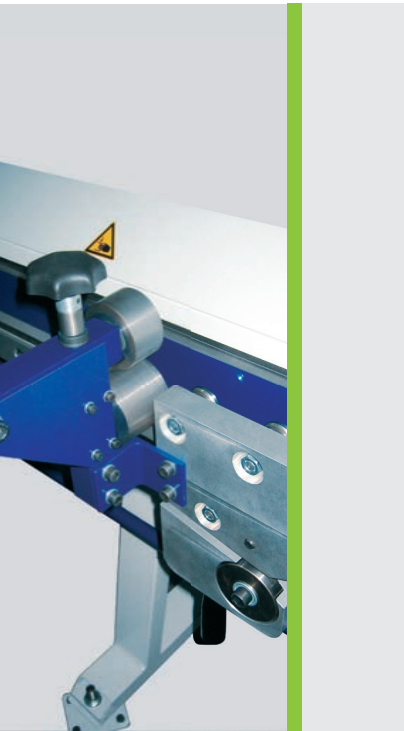
One function of the cutting- and flattening device is to close folding edges
