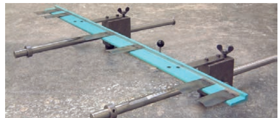
Combined spring finger and back gauge with scale, rack and pinion
