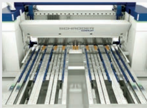
EVO DuoBend with two folding beams
