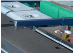
Bottom beam blade with finger grooves
