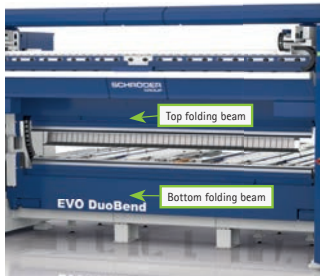
EVO DuoBend with two folding beams
