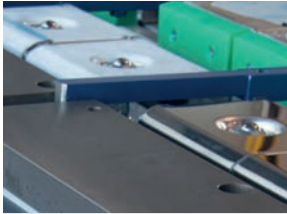
Bottom beam blade with finger grooves
