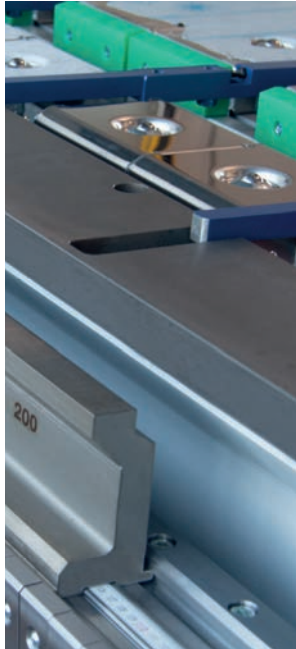
Bottom beam blade with finger grooves and folding blades
