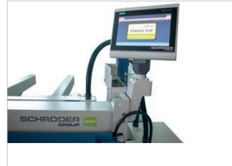
NC positioning gauge Classic Cut with touch control on turnable panel
