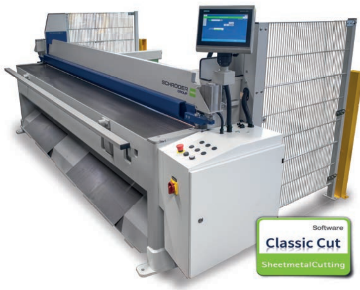
The MSHU with sheet support to the front and the new NC positioning gauge Classic Cut. Working height: 920 mm.
