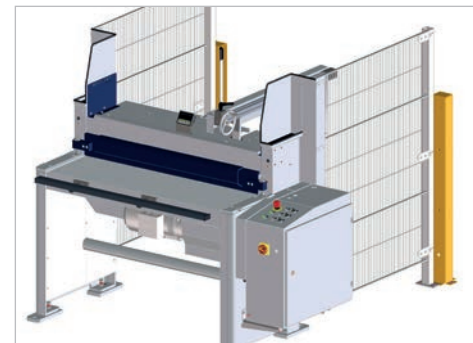
Standard: MHSU with rear guarding via 3-beam light barrier incl. side protection grid and manual back gauge.
