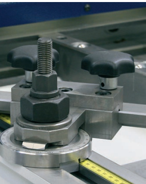
Angle gauge adjustable 0-360° according to scale
